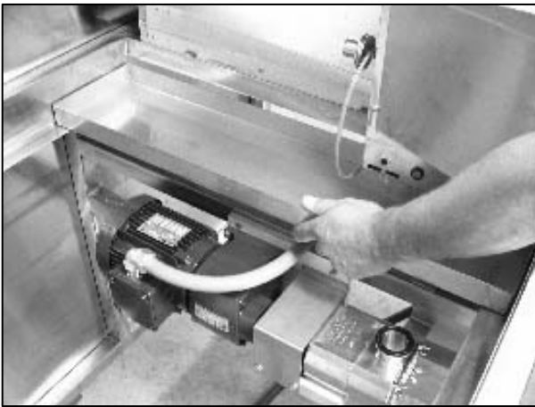
34. Remove the drip pan.
